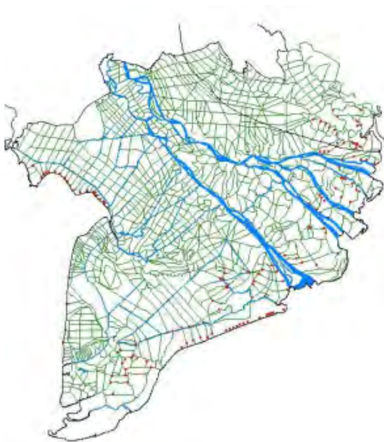
Fig. 3.3 Irrigation Canals and Salinity Control Structures in Mekong Delta, from MRC Irrigation Database (Note: Salinity control structure is shown as a point)
