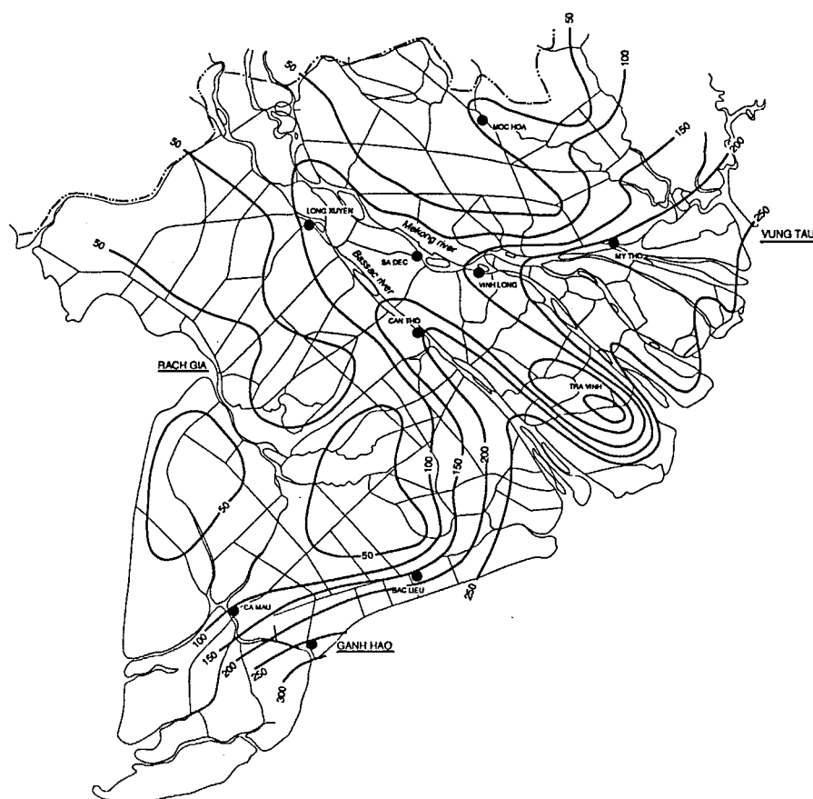
Fig. 3.10 Attenuation of Tidal Propagation in the Mekong Delta
