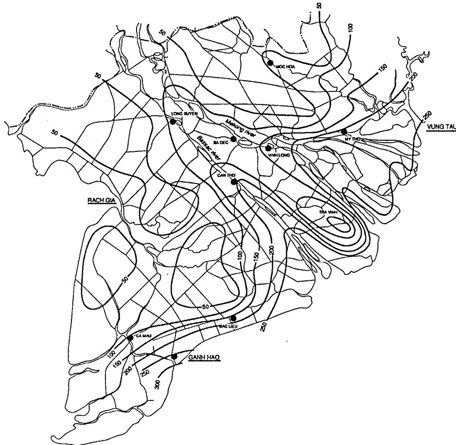
Fig. V-2-11 Attenuation of Tidal Propagation in the Mekong Delta Note: Contour lines mean equal tidal magnitudes in cm.
