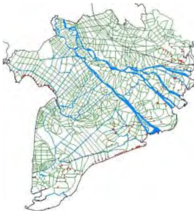
Fig. V-2-5 Irrigation Canals and Salinity Control Structures in Mekong Delta, from MRC Irrigation Database (Note: Salinity control structure is shown as a point.)
