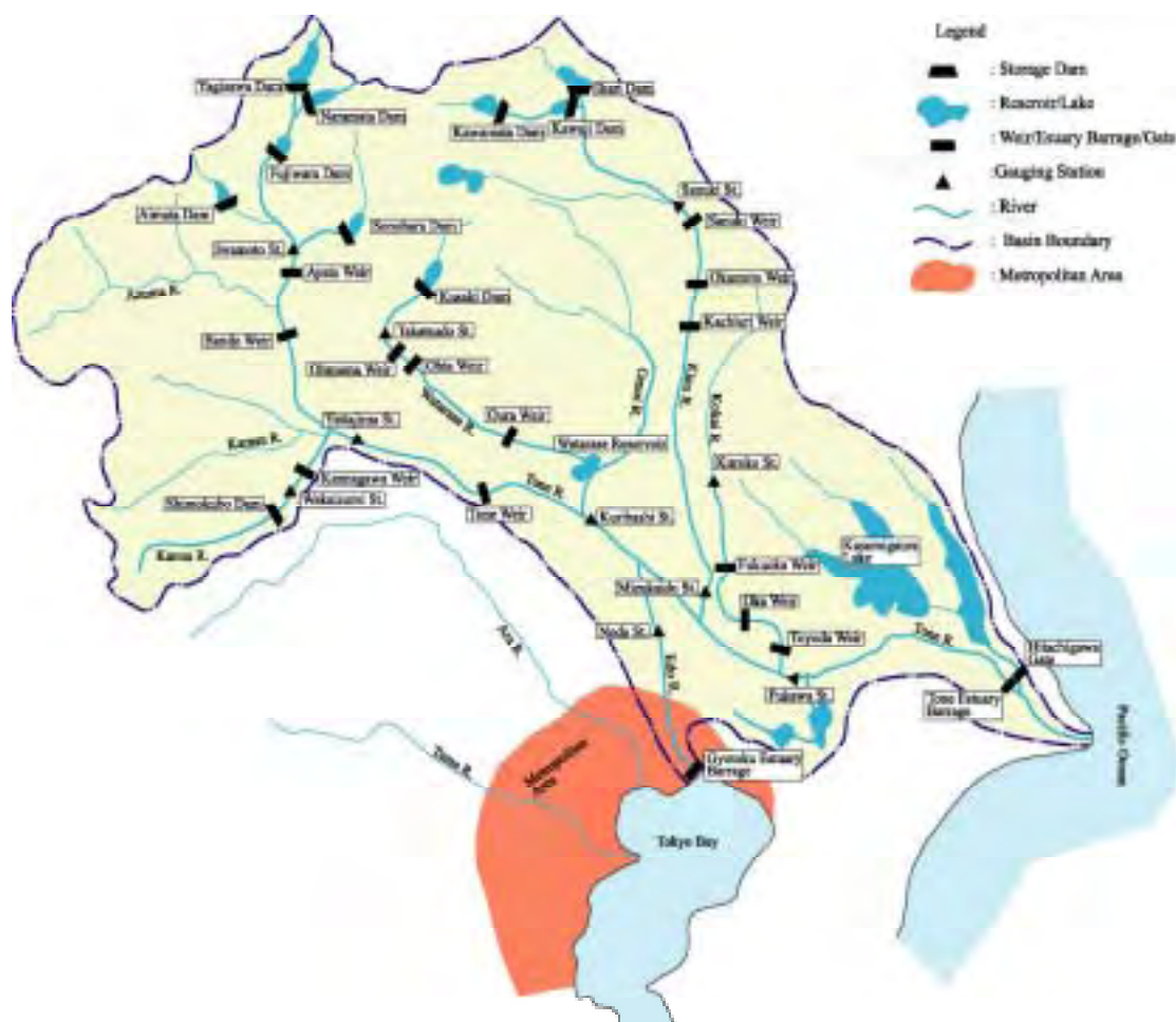
Fig. V-4-9 Major Storage Dam and Intake Sites in the Tone River Basin
