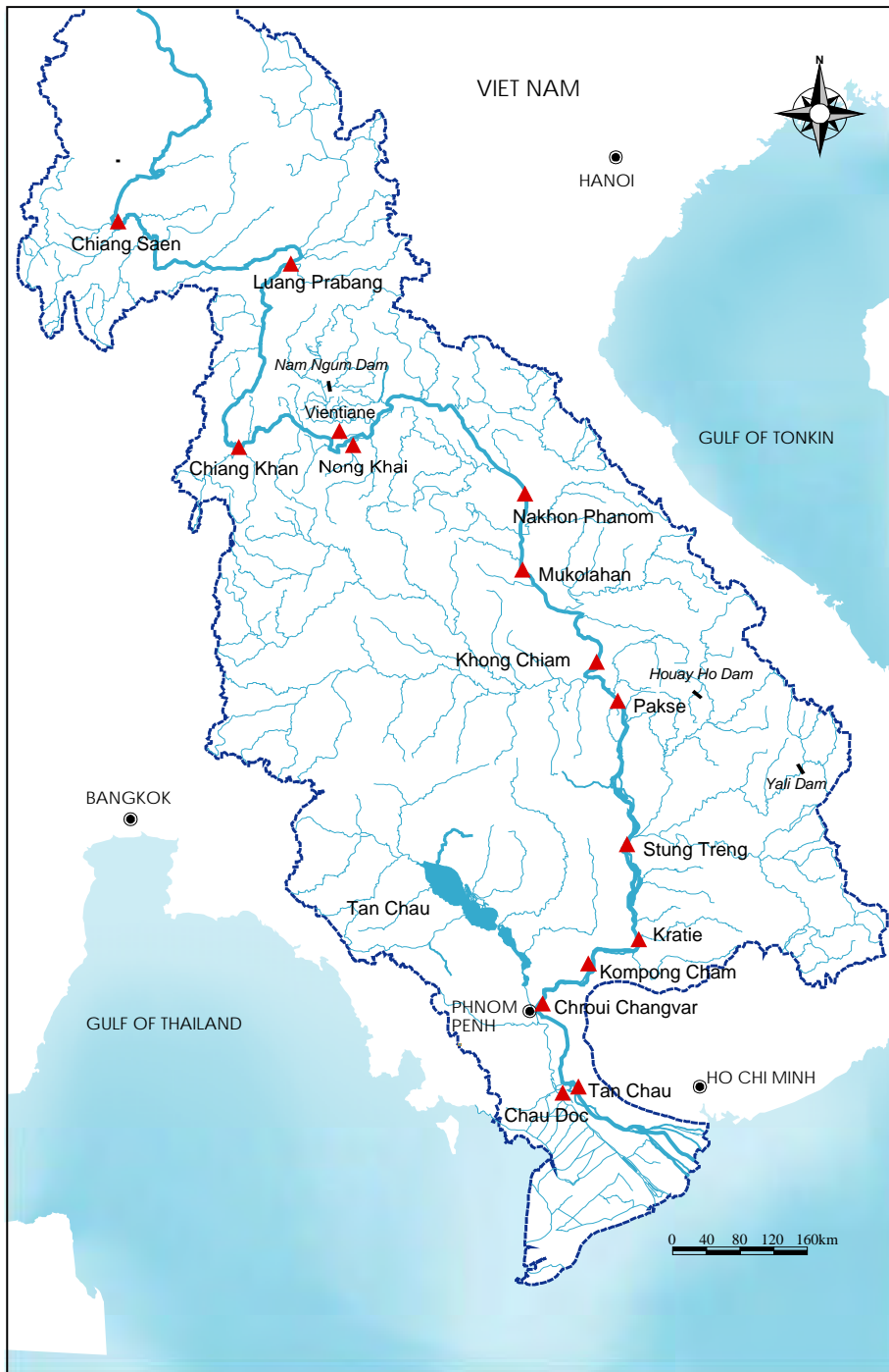
Fig. IV-1-1 Major Hydrological Stations on the Mekong Mainstream
