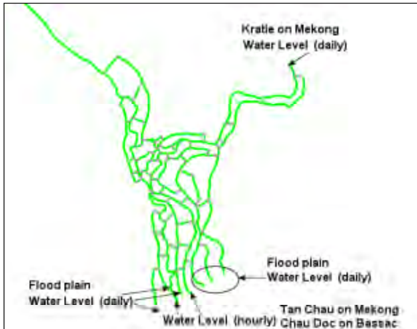
Fig. III-1-17 Locations and Types of Boundary Condition Applied
