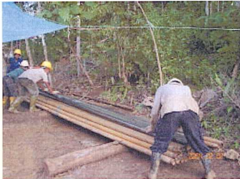
NQ Rods pulled out
