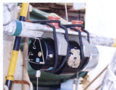
One-shot Deepsea Camera (Installed to MC)
