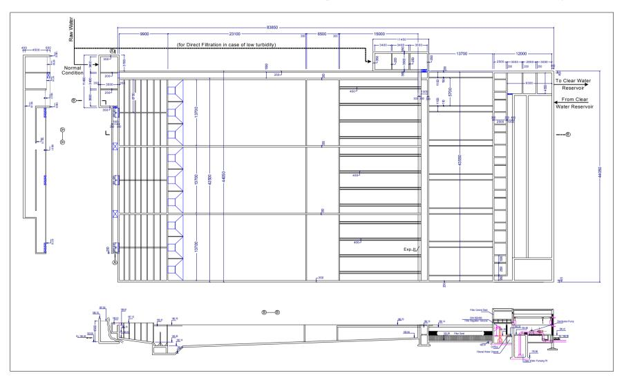
Plan and Section of Flocculation, Sedimentation and Filter in Thangone Treatment Plant Construction: 60,000 m3/day
