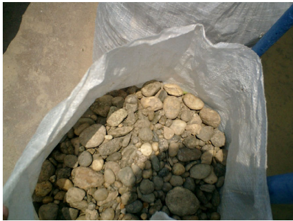
Removed Gravels from Gravel Filter
