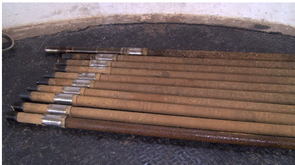
Shafts Extracted from Intake Pump
