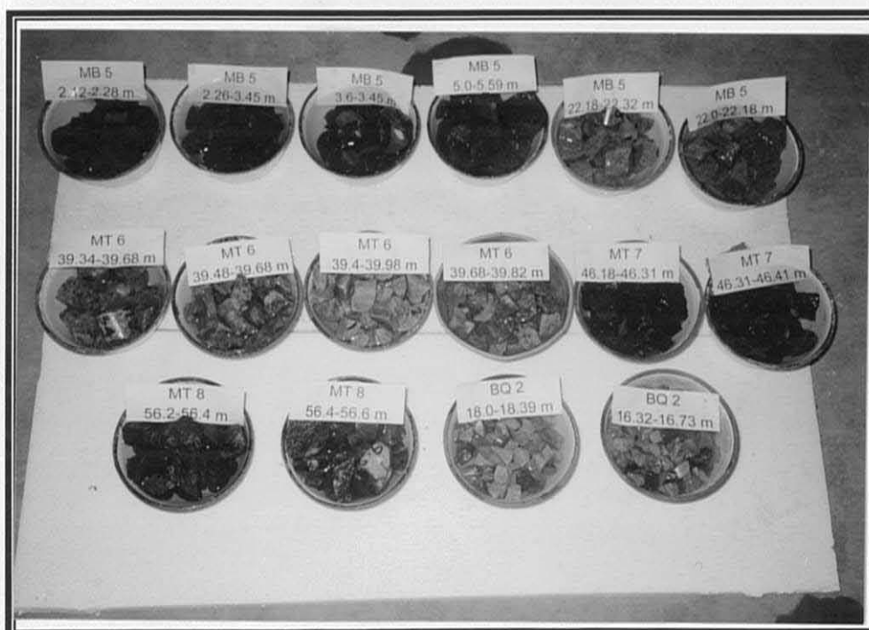
Photograph 8: Core samples used for testing 'specific gravity and water Absorption'
