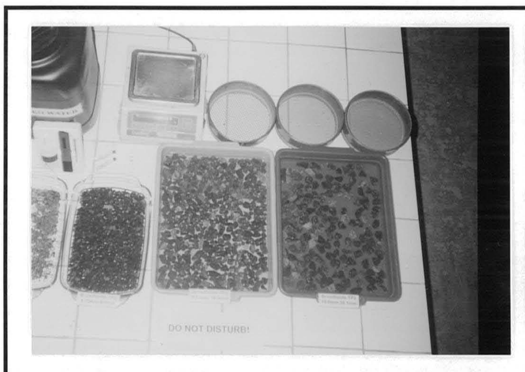
Fig 13 : Clay Lumps and Friable Particles- Test in Progress
