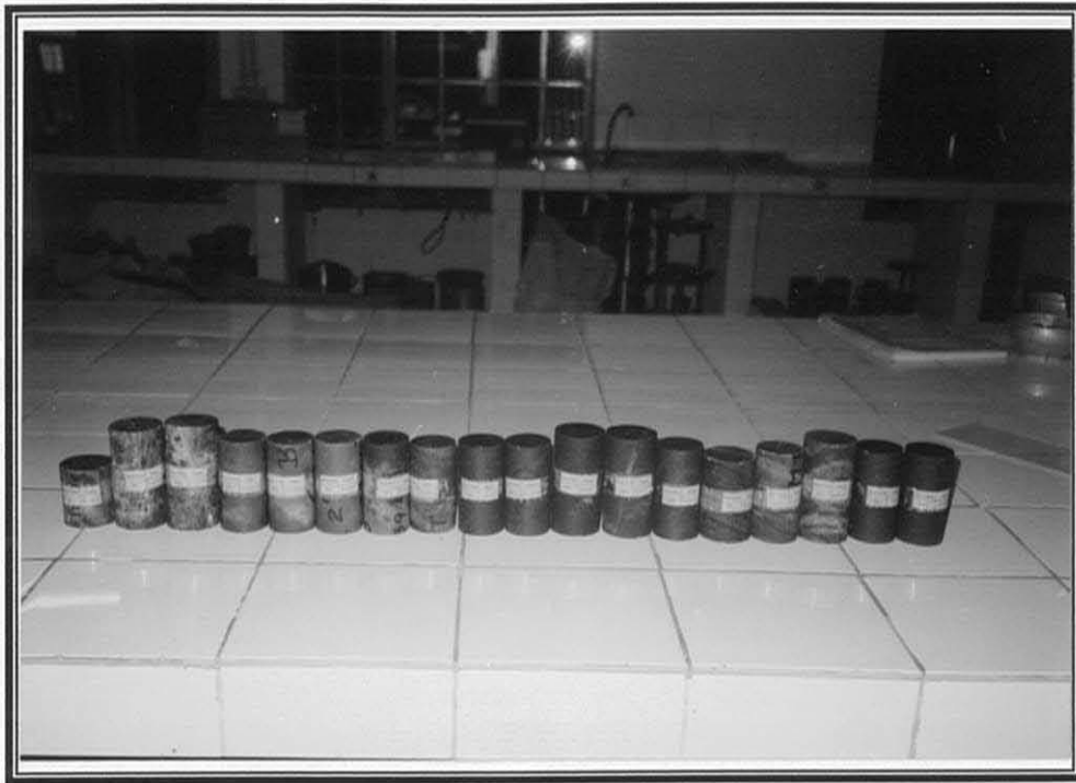
Photograph 9: Core samples used for testing 'unconfined compression' and 'ultra sound wave velocity'
