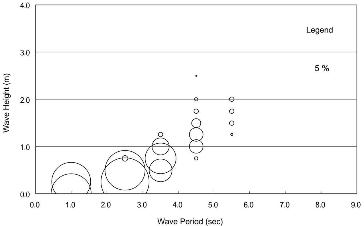
**Figure G-3 Combined Occurrence of Wave Height and Wave Period at Off-Tanjung Priok Port (1997 - 2001)**
