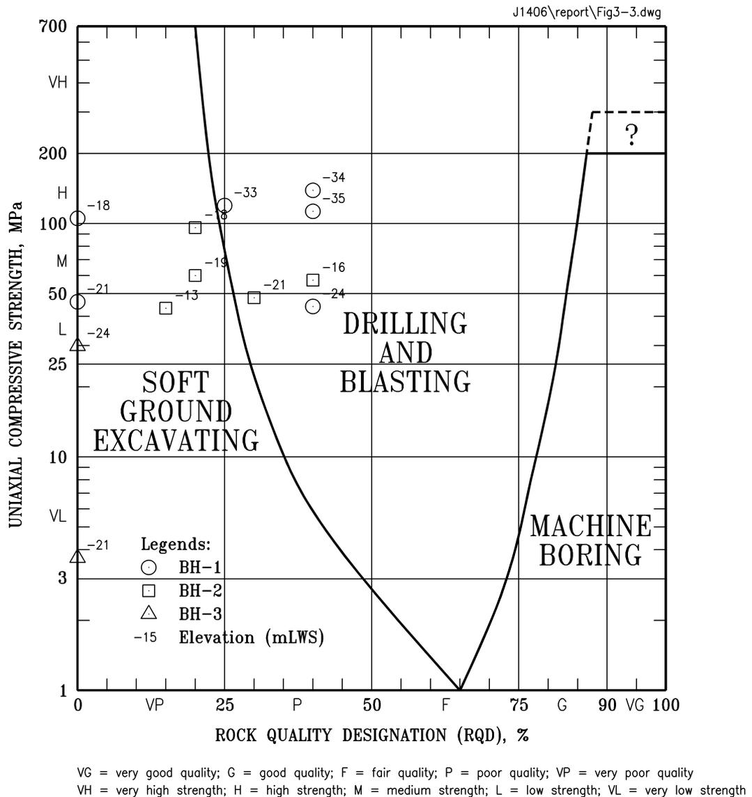
**Figure I-1 Workability of Rock (after Muir Wood, 1972)**
