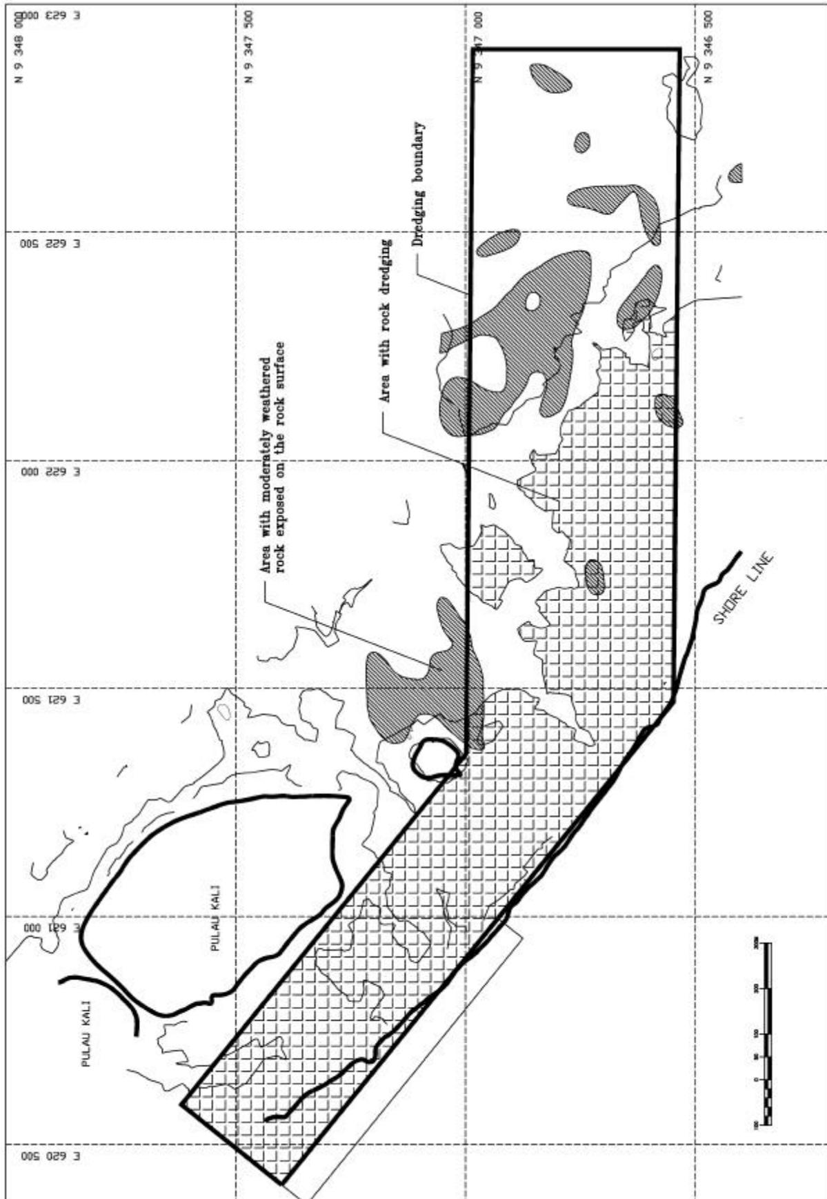
Figure H-1 Bedrock Surface Contours and Anticipated Area of Rock Dredging
