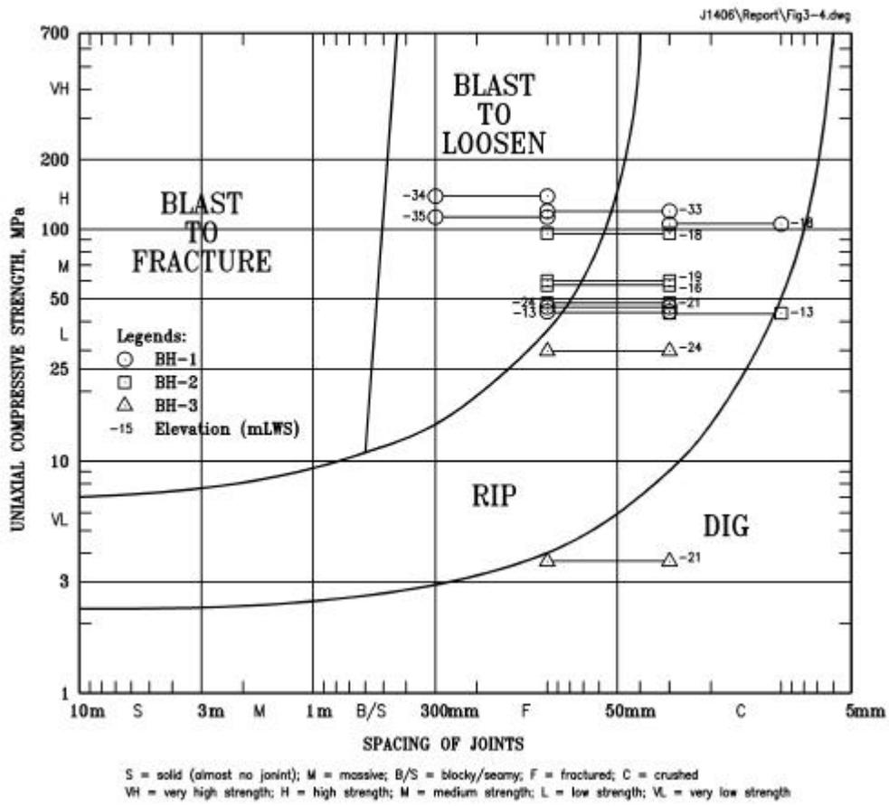
Figure H-3 Workability of Rock (after Franklin et al., 1971)
