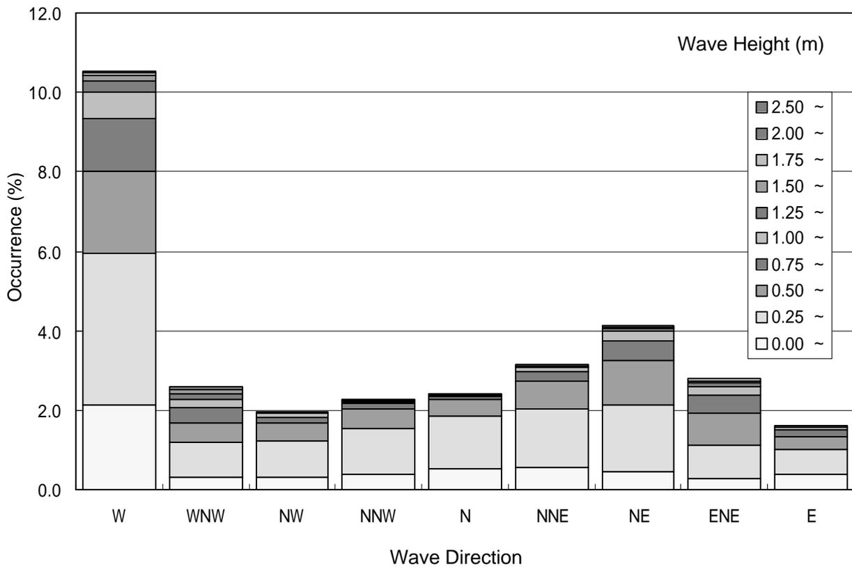
**Figure G-2 Combined Occurrence of Wave Height and Wave Direction at Off-Tanjung Priok Port (1997 - 2001)**
