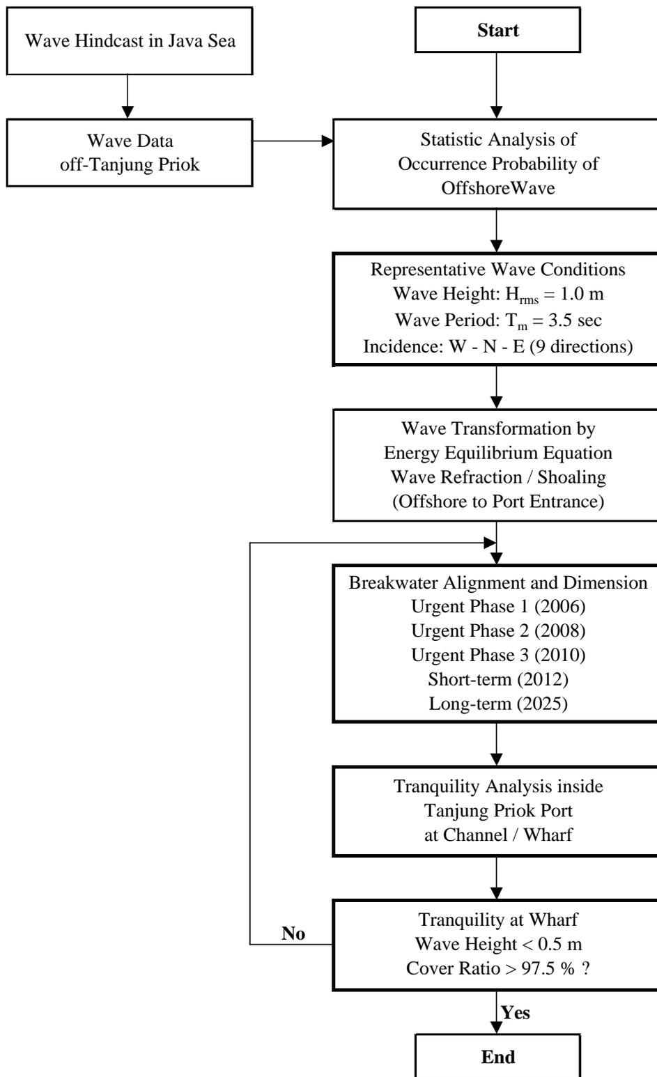
Figure G-1 Study Procedure of Tranquility Analysis and Breakwater Planning
