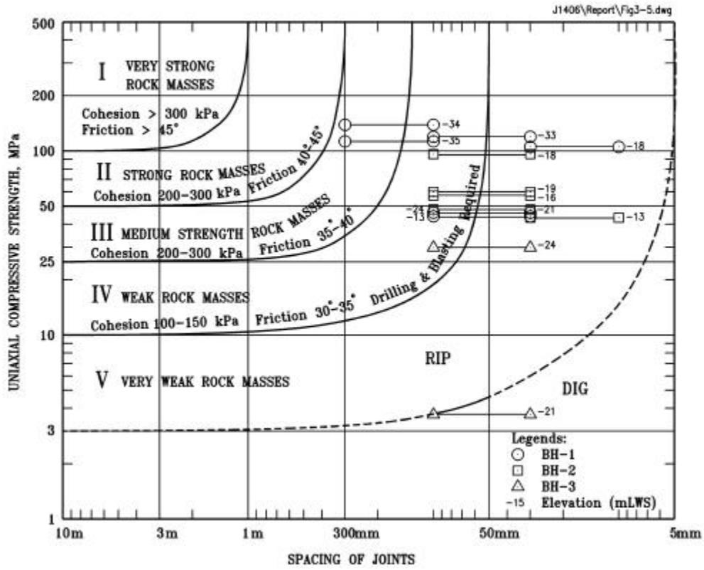
Figure H-4 Strength Diagram for Jointed Rock Masses (after Bieniawski, 1974)
