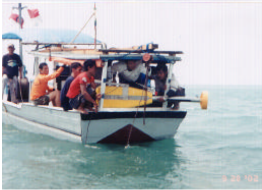
Figure 2-1-19 “Tow Fish for Seismic Reflection Survey, Bojonegara”
