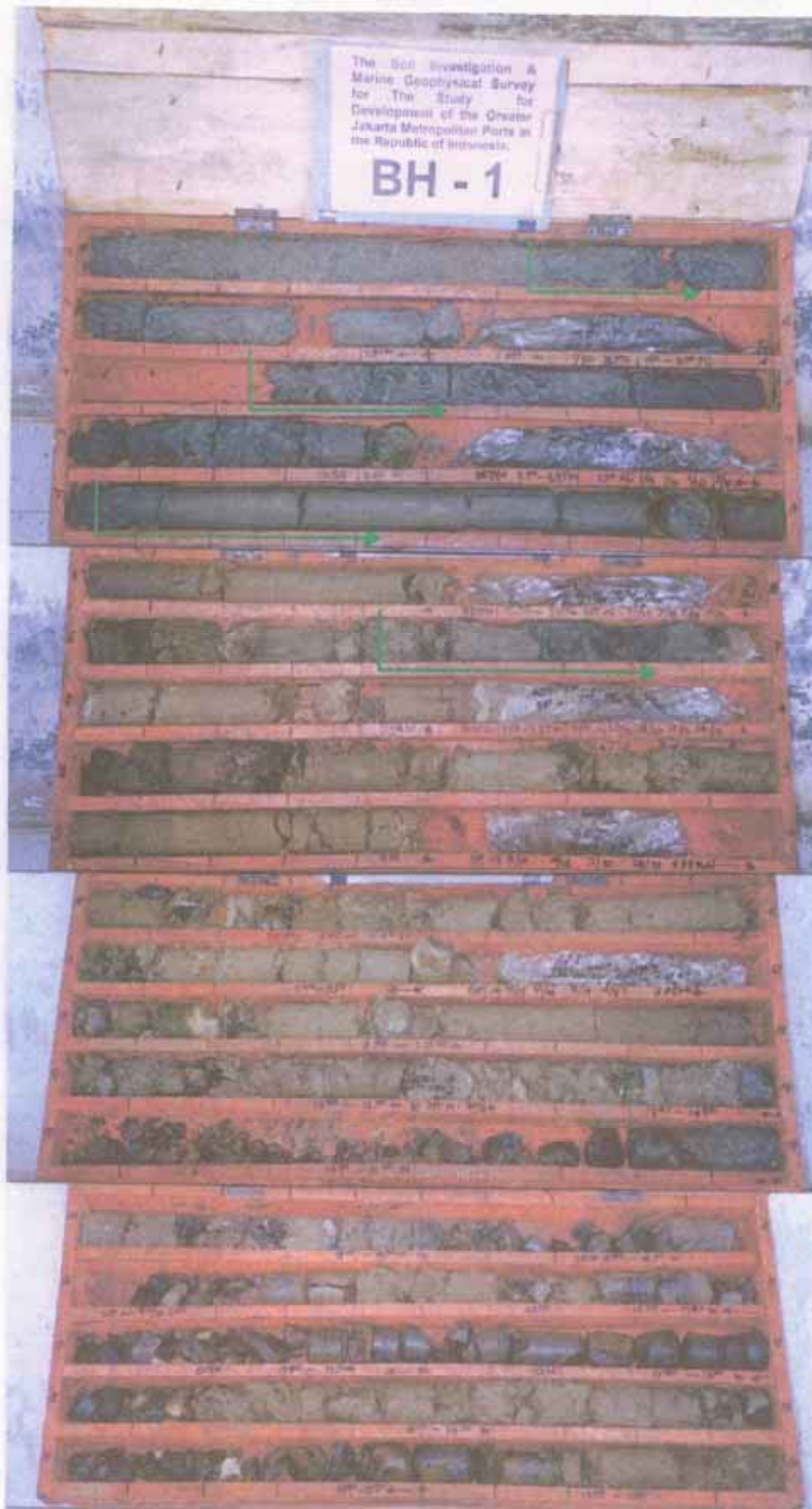
Core Box of Borehole BH-1 (0 - 20m)
