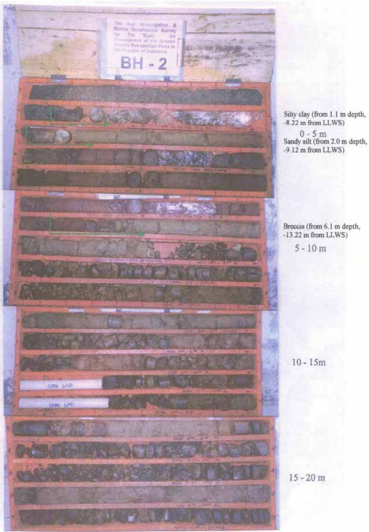
Core Box of Borehole BH-2 (0 - 20m)
