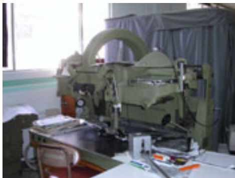
Photo 3.3-1 Analog plotter installed in Photogrammetry Division
