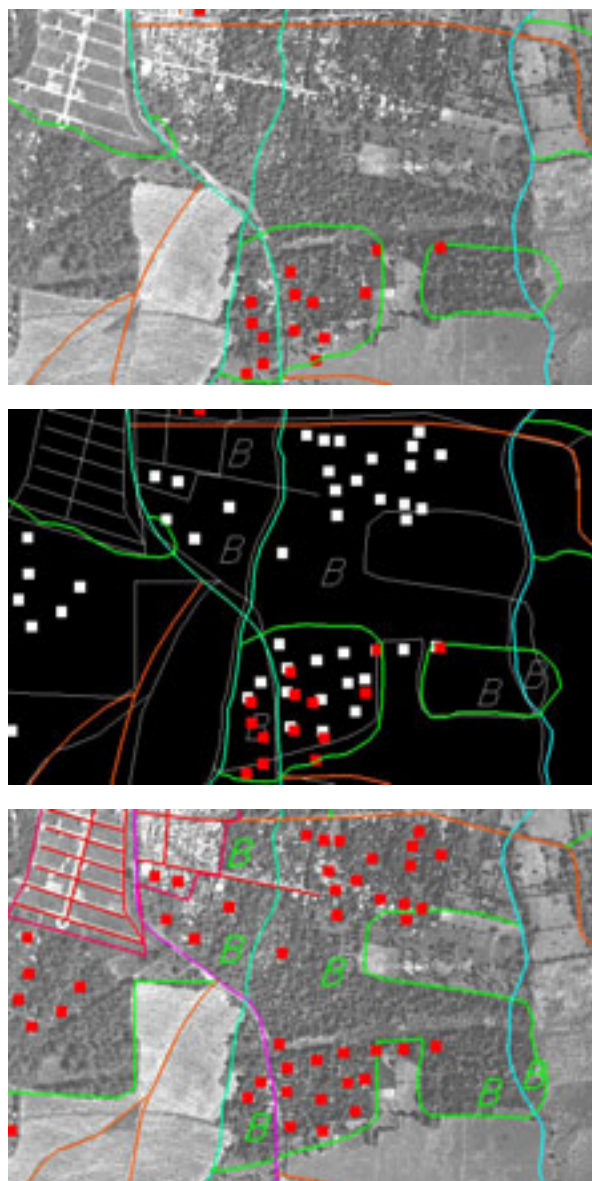
Figure 2.4-12 Existing data + ortho, existing data + new line data, compiled line data + ortho
