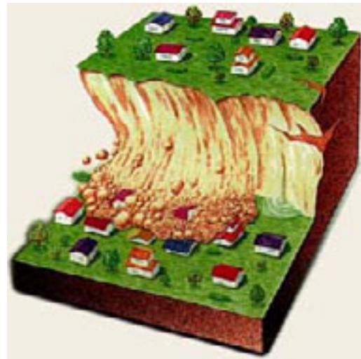
Figure 2.3.8-50 Influence of Slope Collapse on Houses under Cliff (Home page of Ministry of Land, Infrastructure and Transport of Japan)
