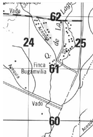
Figure 2.1-51 Coordinate values on grid lines and their positions on printed map
