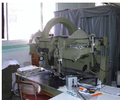
Photo 6.2-1 Analog plotter installed in Photogrammetry Division
