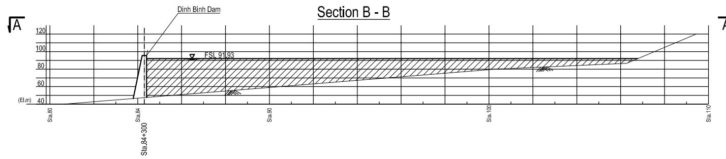
Typical Cross Section of Non-overflow Section
