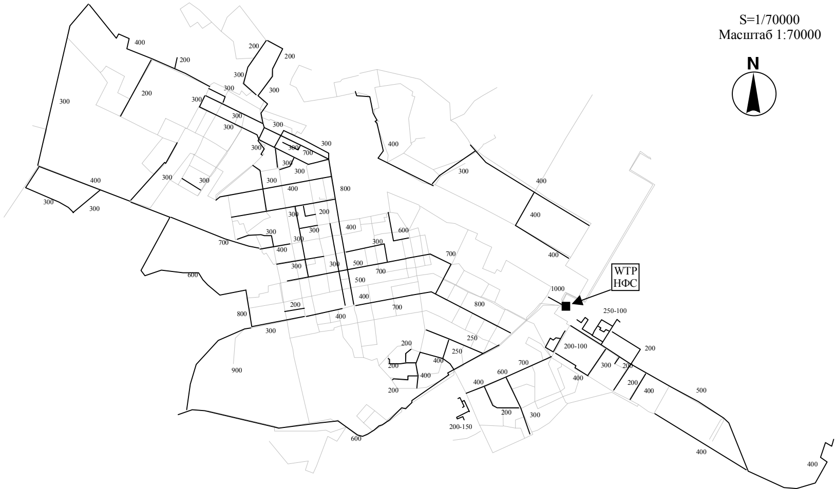
Figure 5.4.2 Location of Pipes to be Replaced
