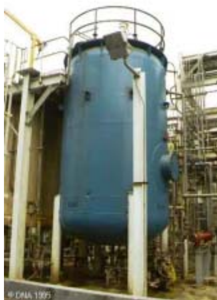
Figure 6.3.15 Example of Continuous Neutralisation / Precipitation Reactor
