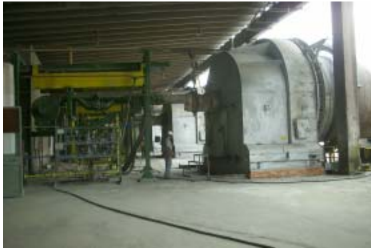
Figure 4.1.2 Blended Waste Feed System at Cement Kiln
