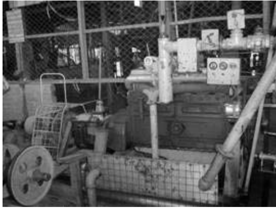
Fig.1 Rice Mill Engine Powered with Husk Gas
