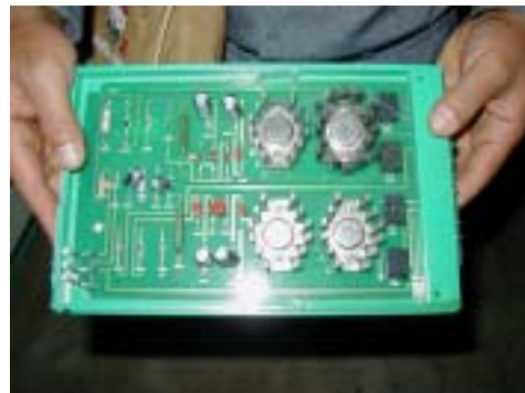
Damaged board of Thyristor controller
