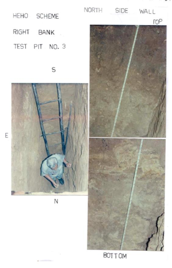
Figure B-5-23 Photograph of Right Bank Test Pit No.3 (1/2)
