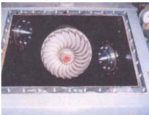
Figure 3.4 Inner Shape of Turgo Impulse Turbine
