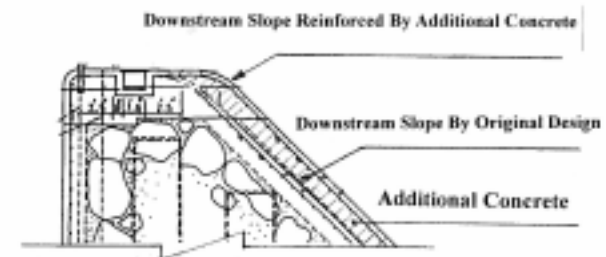
Weir Body Reinforced By Additional Concrete
