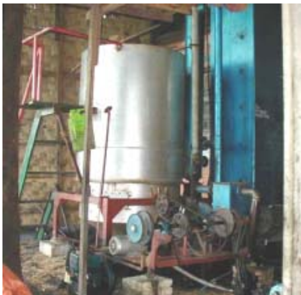
Gasifier tank (above), husk feeding to the tank (top right), and the entire system (bottom right).
