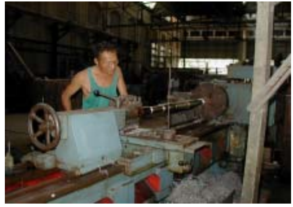
Making shaft for Crossflow turbine
