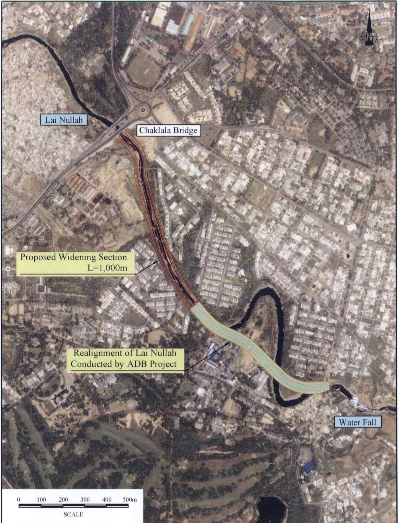
Fig. 6.2.5 Proposed Widening Section of Lai Nullah below Chaklala Bridge
