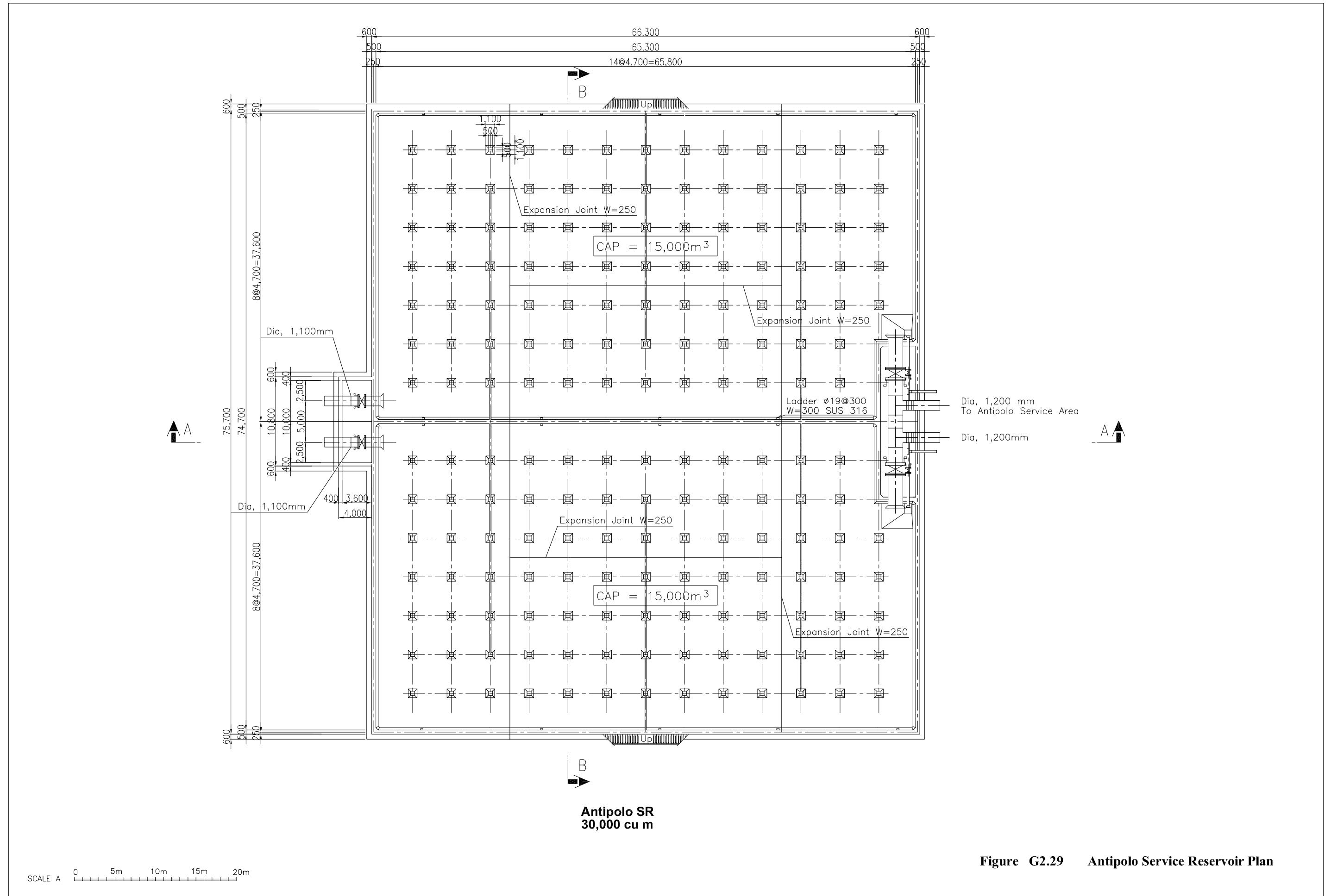
**Figure G2.29 Antipolo Service Reservoir Plan**
