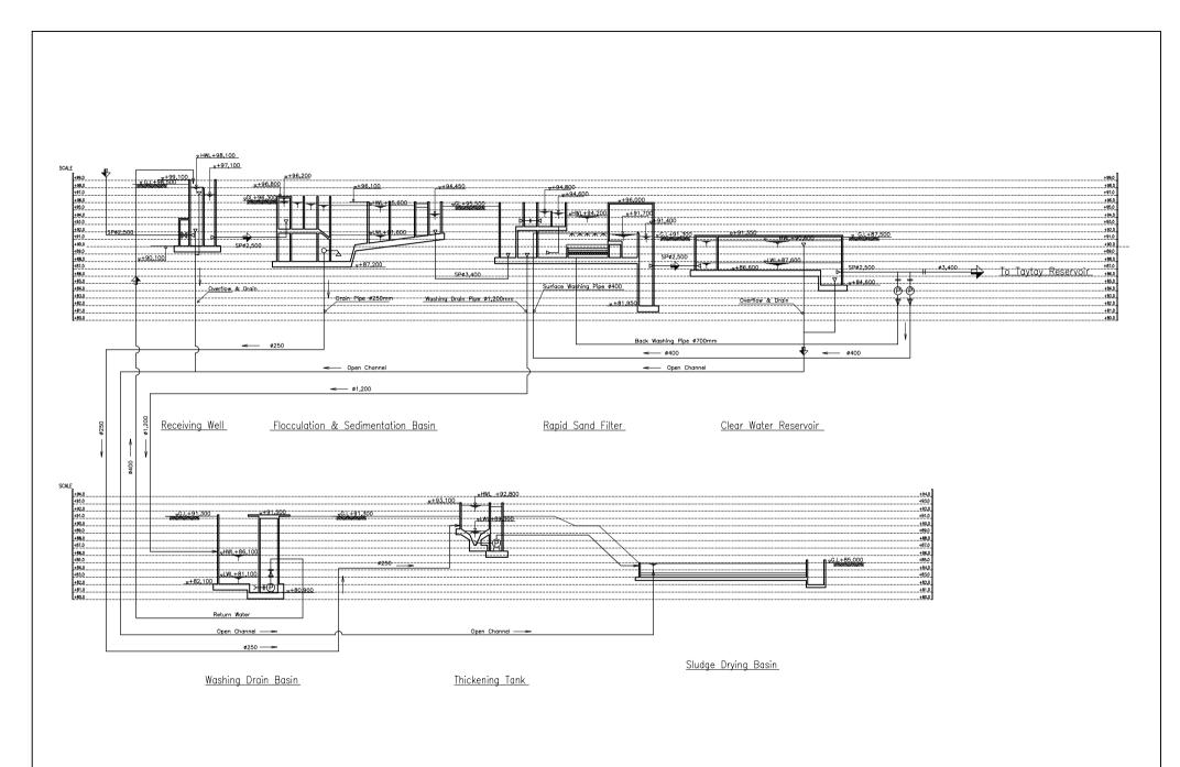
Figure 7.6 Hydrauric Profile of Morong Water Treatment Plant
