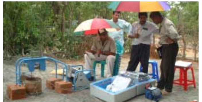
WRB engineers who conduct well logging using donated equipment.
