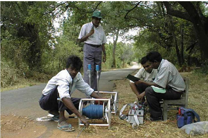
WRB engineers who conduct Electrical Resistivity Survey (Schlumberger method) by using donated equipment.
