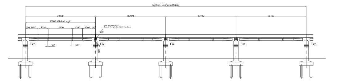
Plan (1 Span of 30m Length) Scale 1:250
