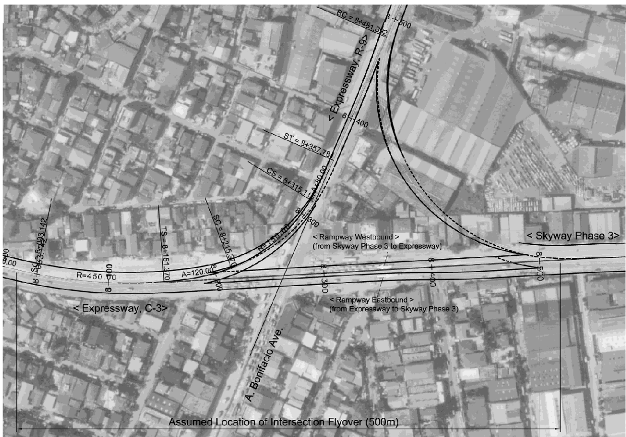
Figure 4.19 Expressway Alignment and Location of Planned Intersection
