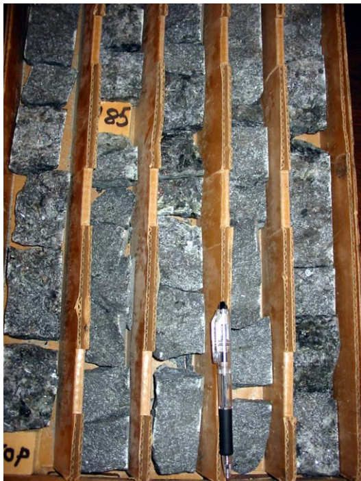
Wetlegs deposit, Unit I (D.H. W-8B): heterogeneous sulfide-bearing augite troctolite (Cu:0.25-0.34%, Ni:0.07-0.10%).
