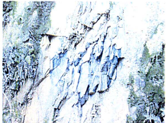
Photo-2 : Pelitic schist. N45E, 73SE trending Schistosity. \kappa = 0.19 (Susceptibility \times 10^{-3} emu/cc).
