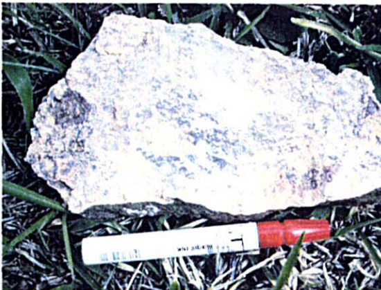
Photo-5 : Castro Fm. (Ordovician). Weak altered tuff breccia. \kappa = 0.59 .
