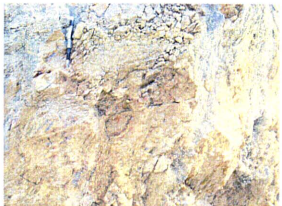
Photo-4 : Limestone in Abapa quarry (Proterozoic) N50E, 52SE. \kappa = 0.63 .
