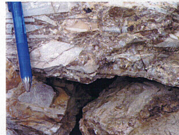
Quartz fills in the country rock (sediments) with pyrite and green copper mineral.
