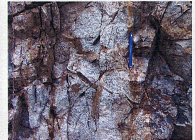
Occurrence of silicification and K-alteration (biotitization) in porphyry (dacitic).
