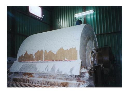
11. Sludge from the rotary filter (Esfahan)
