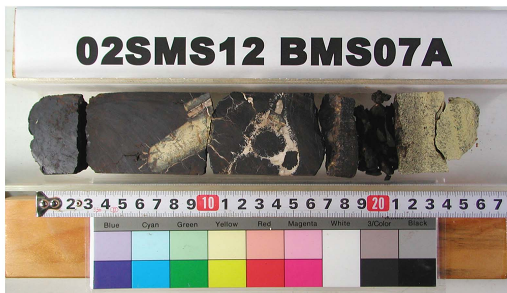
Drill. Len. 29cm, Thick. Sedim. 3cm, Core Len. 26cm, Crust 18cm
