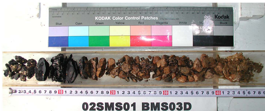
Drill. Len. 162cm, Thick. Sedim. 0cm, Core Len. 45cm, Crust 13cm
