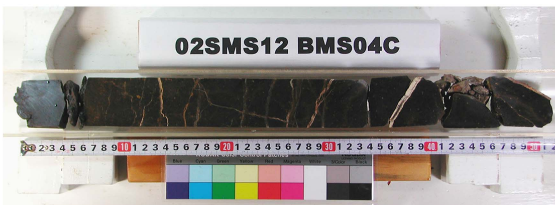
Drill. Len. 65cm, Thick. Sedim. 15cm, Core Len. 50cm, Crust 6cm
