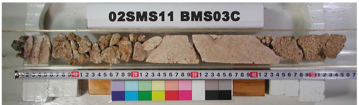
Drill. Len. 107cm, Thick. Sedim. 15cm, Core Len. 55cm, Crust 0cm
