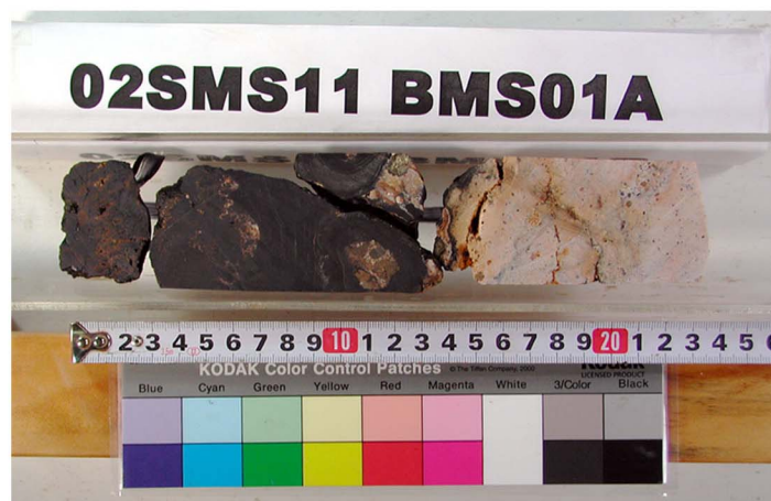
Drill.Len. 26cm, Thick.Sedim.1cm, Core Len.23cm, Crust 9.5cm, Nodule 1cm
