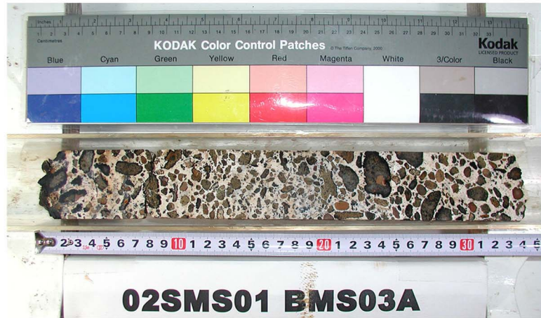
Drill. Len. 49cm, Thick. Sedim. 15cm, Core Len. 34cm, Crust 0.3cm
