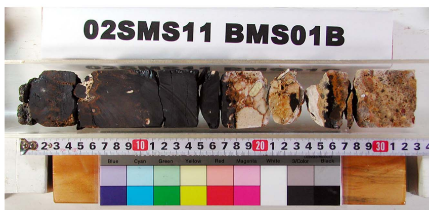
Drill.Len. 34cm, Thick.Sedim.0cm, Core Len.32cm, Crust 16cm
