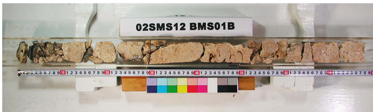
Drill. Len. 82cm, Thick. Sedim. 5cm, Core Len. 77cm, Crust 0cm
