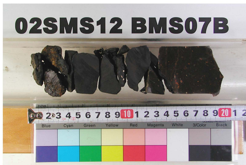
Drill. Len. 20cm, Thick. Sedim. 0cm, Core Len. 19cm, Crust 10cm
