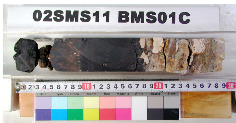
Drill.Len. 33cm, Thick.Sedim.0cm, Core Len.28cm, Crust 16cm
