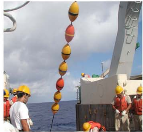
Float of Wire for BMS Operation
