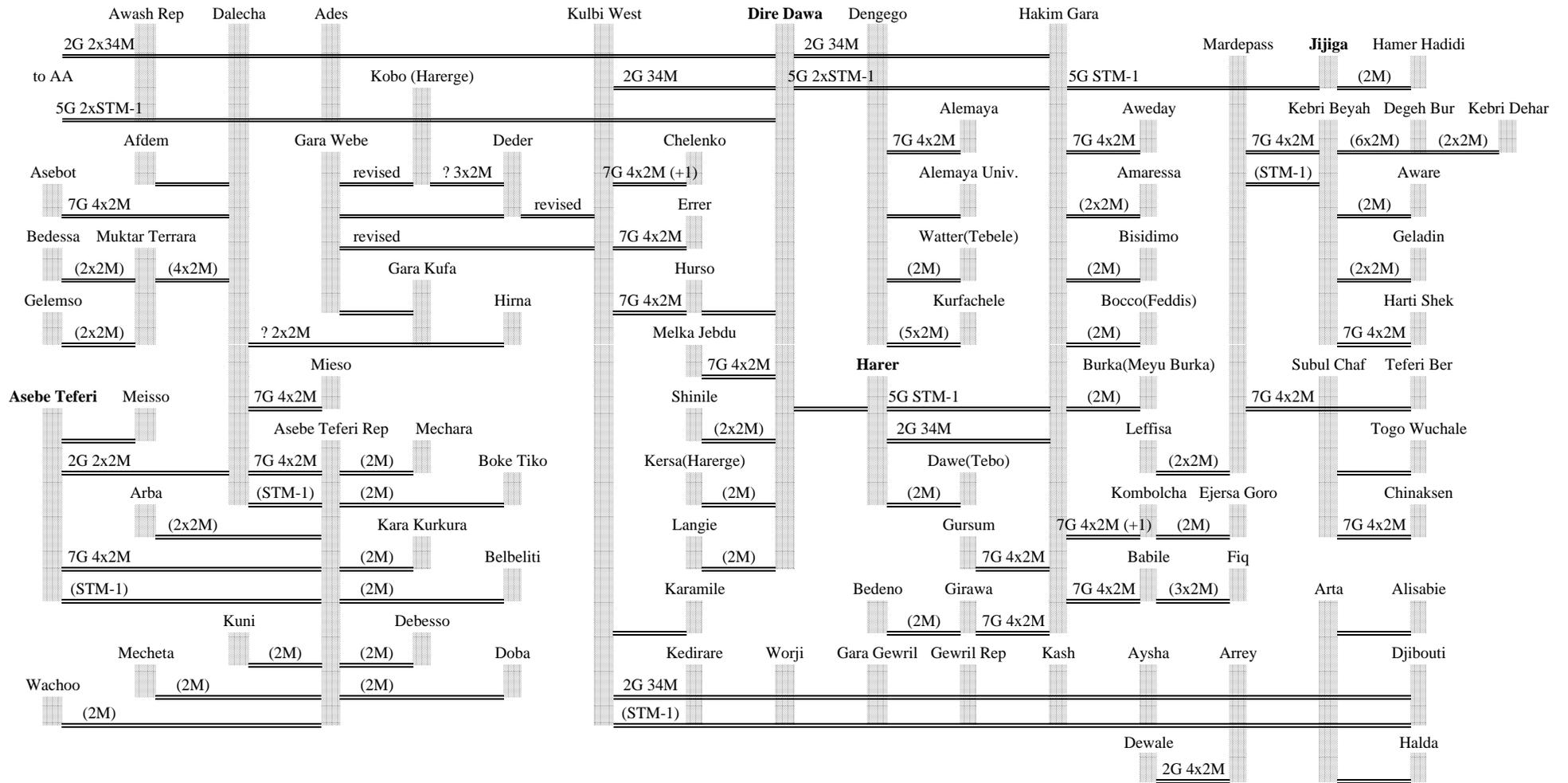
D.Figure9.8-1 TRANSMISSION NETWORK STRUCTURE (Area-05)
