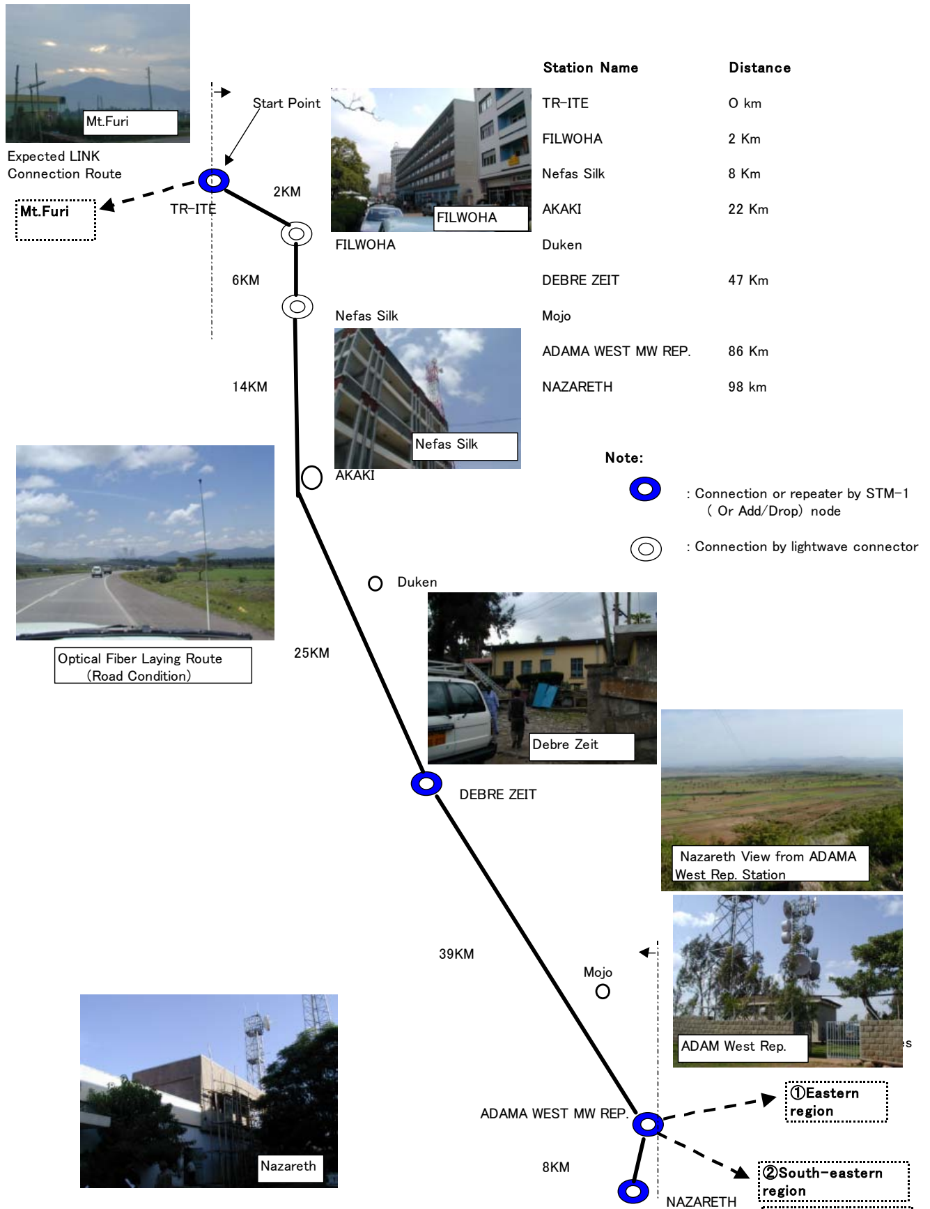
Fig.5.3.1 Transmission Configuration of AA – Nazareth Optical Backbone
