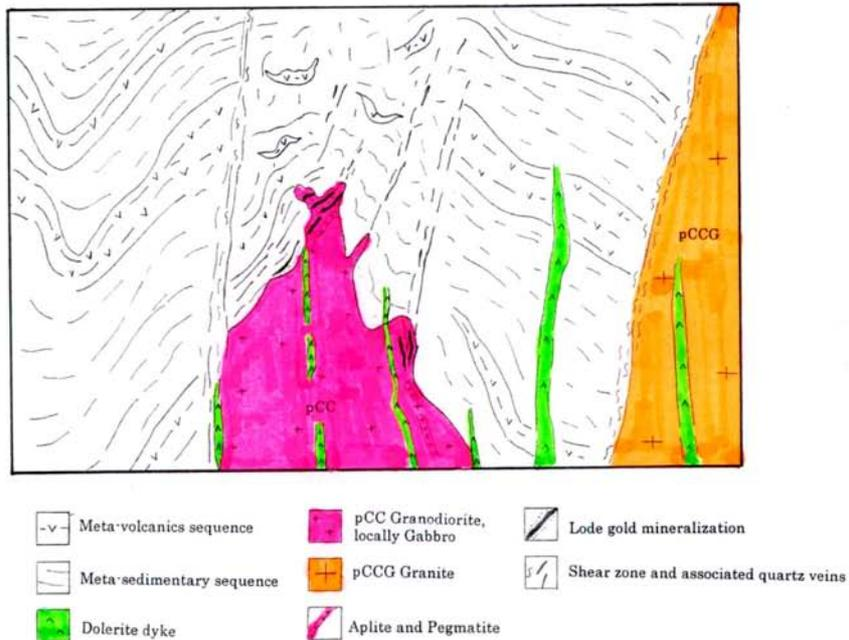
Fig. II-3-9 Schematic model of gold mineralization in San Jose and Arroyo Grande area
