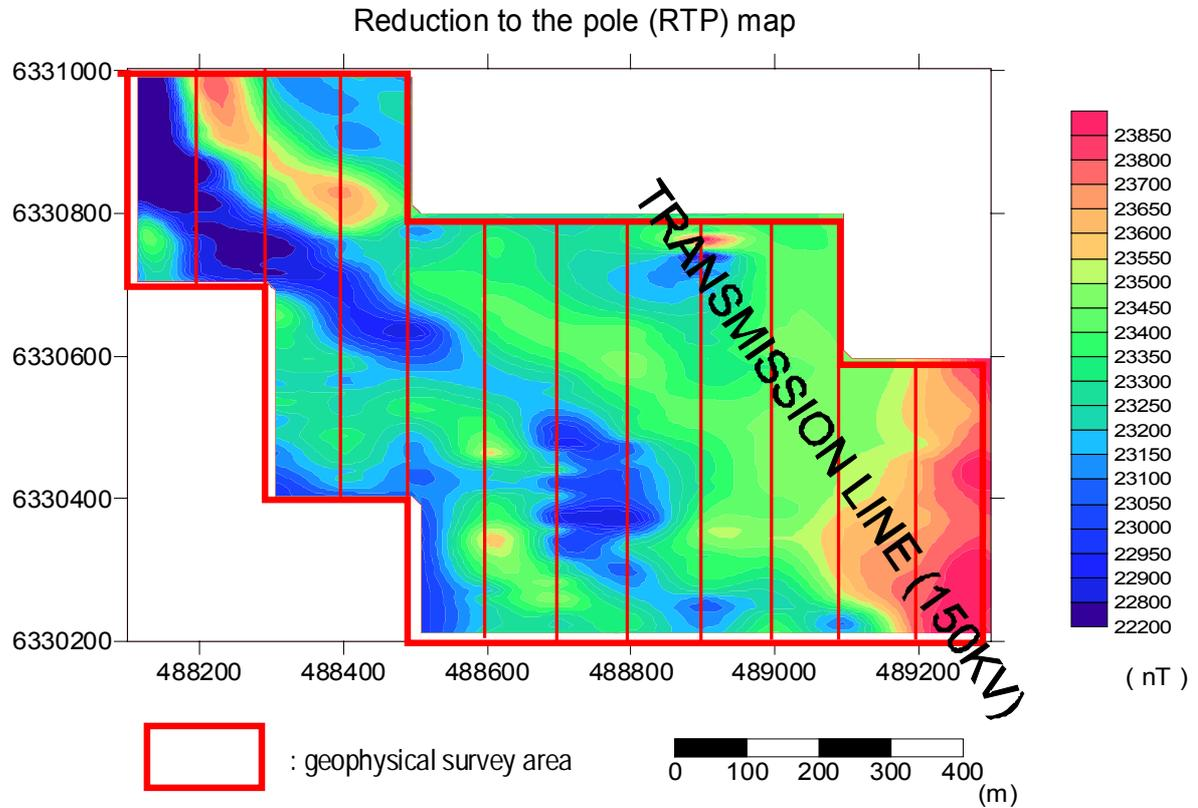
Fig. II-3-14 Total magnetic intensity and Reduction to the pole
