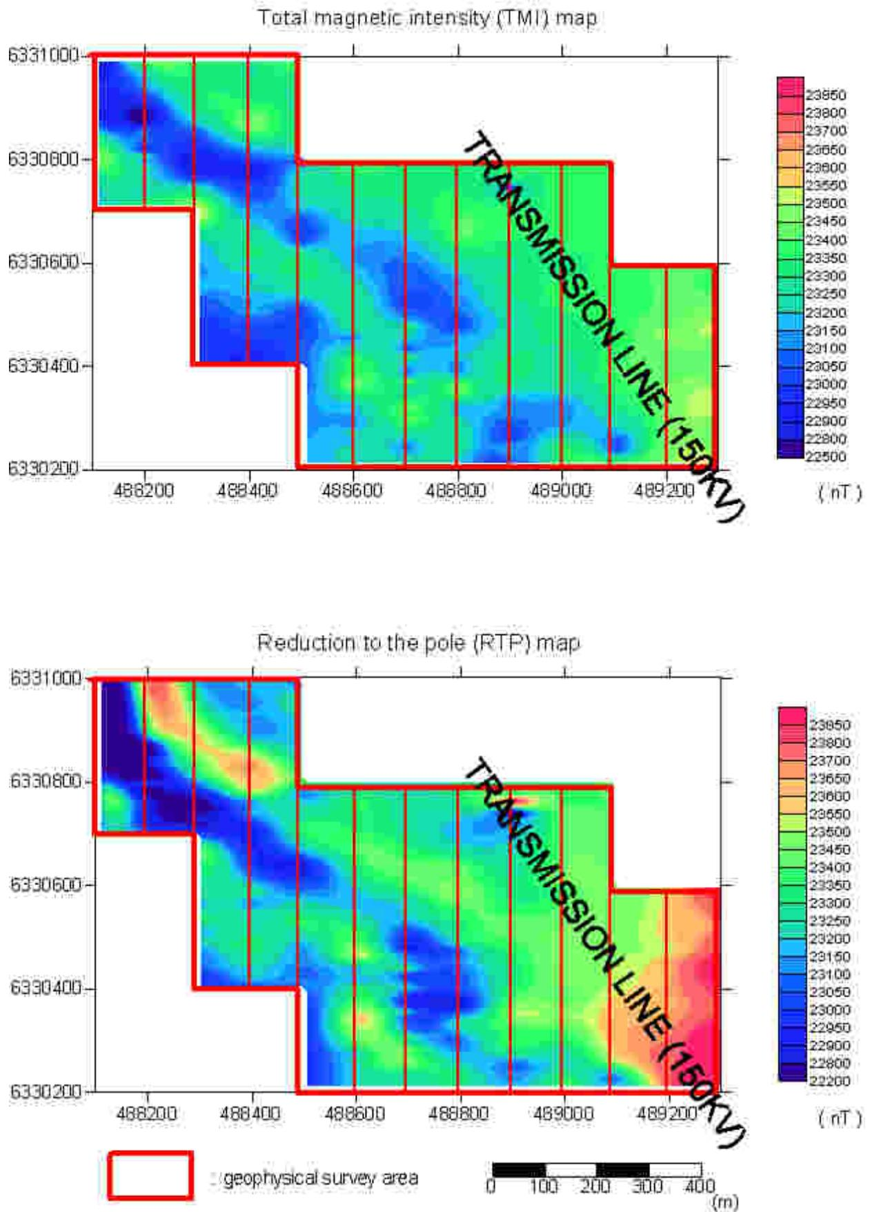
Fig II-6-7 Total magnetic intensity and Reduction to the pole in Andresito East area
