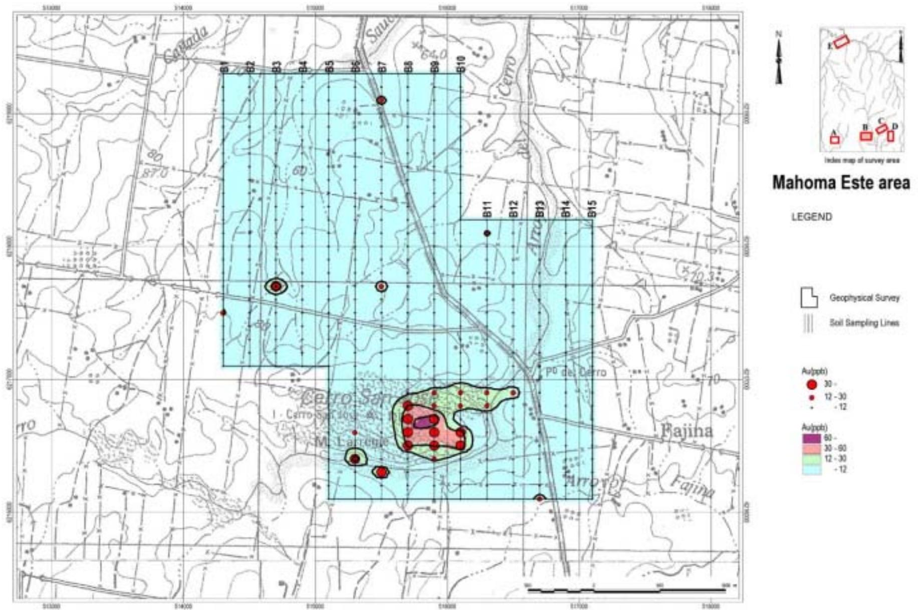
Fig. -5-4 Result of soil geochemical survey in Mahoma Este area
