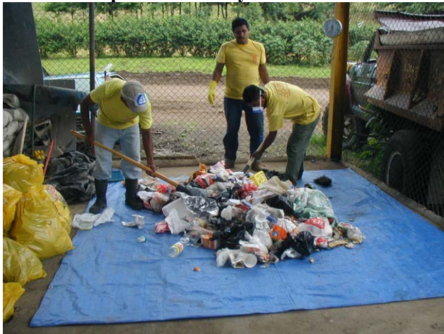
Thorough mixing of collected waste samples
