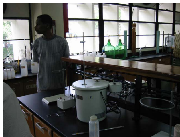
Lower calorific values of wastes were analyzed by using bomb calorimeter
