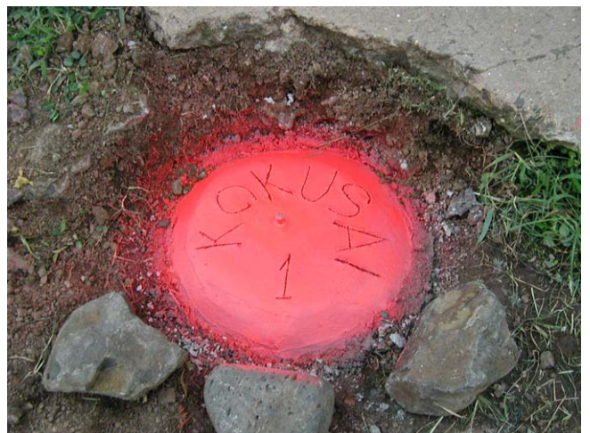
Control points were established in the Cerro Patacon Site
