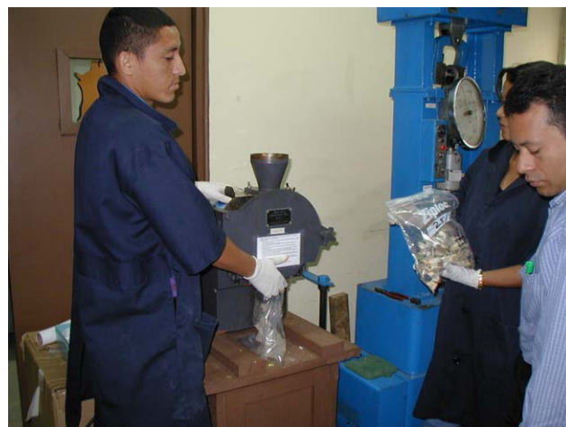
Waste was grinded for chemical analysis
