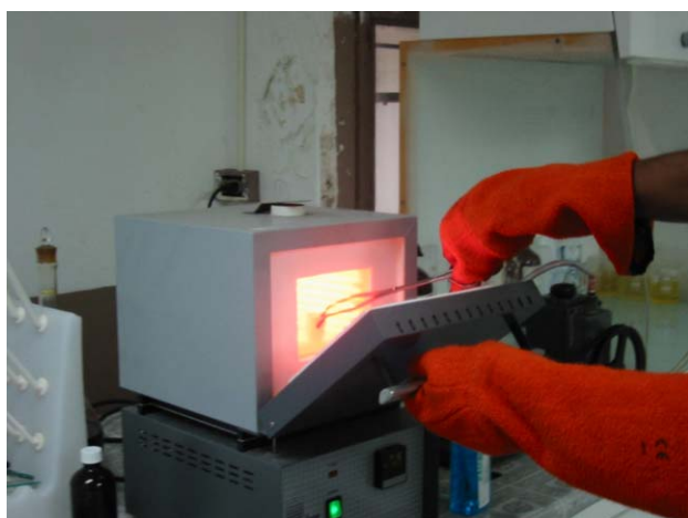
Ash contents and volatile solids were analyzed by burning samples
