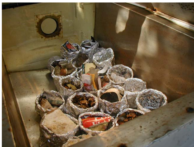
The components were dried to analyze their moisture contents
