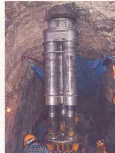
Plate Loading Test (Loading Plate and Testing Equipment )
