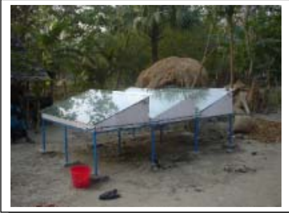
Before and after installation. Site for basin type solar distillation unit Near tube well no. 20
