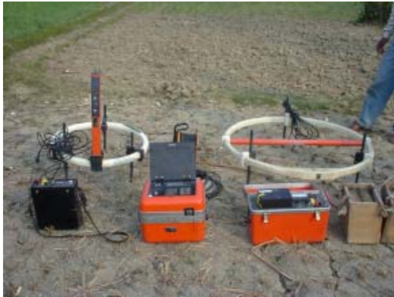
TEM47 Coil TEM57 Coil TEM47 Transmitter Receiver Protem57(D) TEM57 Transmitter
